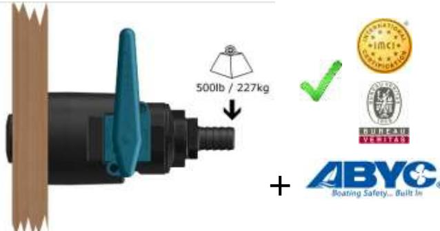
In accordance with ISO 9093-2 standards, Skin Fittings (Thru Hulls) are subjected to a 155kg (341.7lb) load, applied to the threaded section for a minimum of 30 seconds, without any damage occurring. TruDesign Skin Fittings (Thru Hulls) meet this standard.
