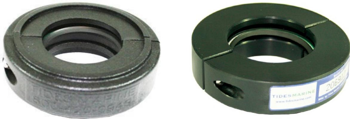
Tides Marine Spare Rudder Seal Carriers were developed as a convenient place to store spare lip seals on the rudder stock. The unit also makes the job of replacing the lip seal in a Tides Marine rudder port easier and is recommended as an accessory for all Tides Marine rudder ports. Installed at the same time as the RPB, they allow the lip seal to be replaced without uncoupling the rudder stock from the steering system or dropping the rudder.
