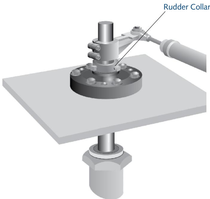
Tides Marine Rudder Collars are for use on power boats. Machined from 304 stainless steel, each unit comes with two threaded locking screws. A third "indexed hole" (which is not threaded) is machined into each Rudder Collar and may be used as a guide to drill "dimples" in the rudder stock. Simply measure your rudder stock diameter (.000") and select the matching part number below.
